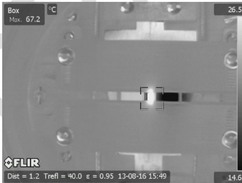
Figure 4-7. The Exit Slit of the Monochromator as Imaged by the FLIR GF320
